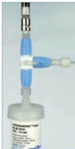
Liquid injection via syringe and 3-way valve
