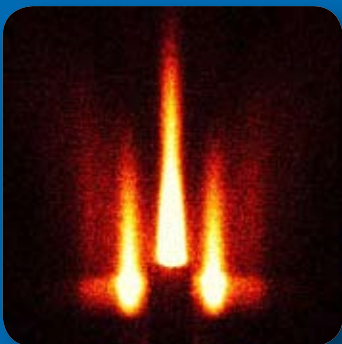
GISAXS pattern of a nanostructured surface
