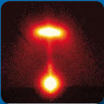
GISAXS pattern of an unaltered multilayer mirror
