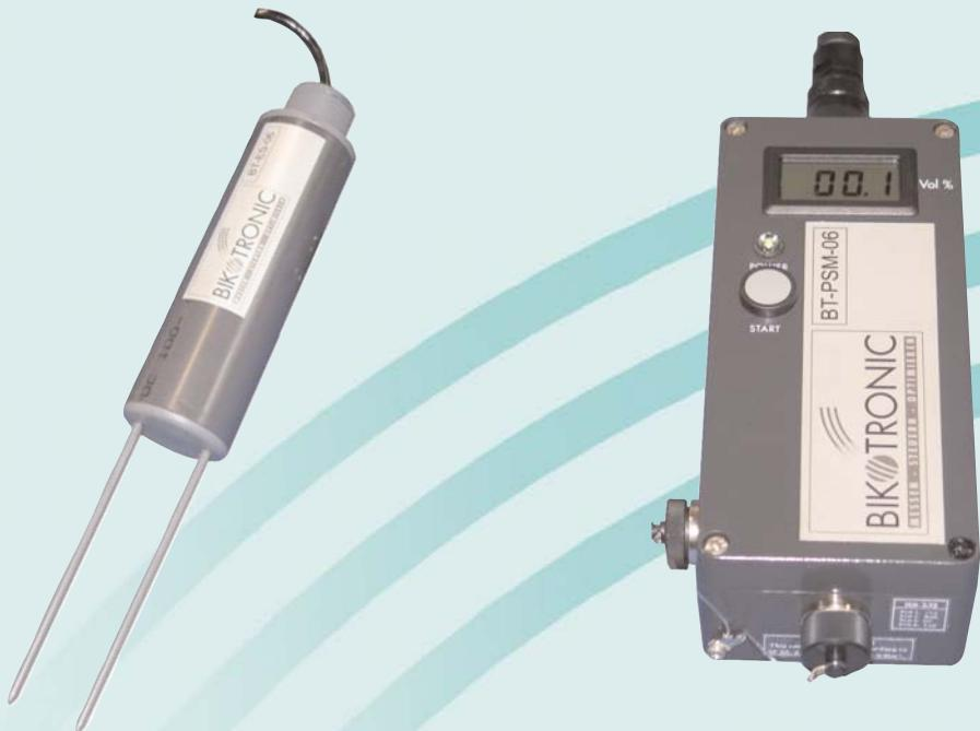
The BT-PSM-06 is the ideal measuring instrument to determine the moisture content in sand and other aggregates fast and precisely on site.
