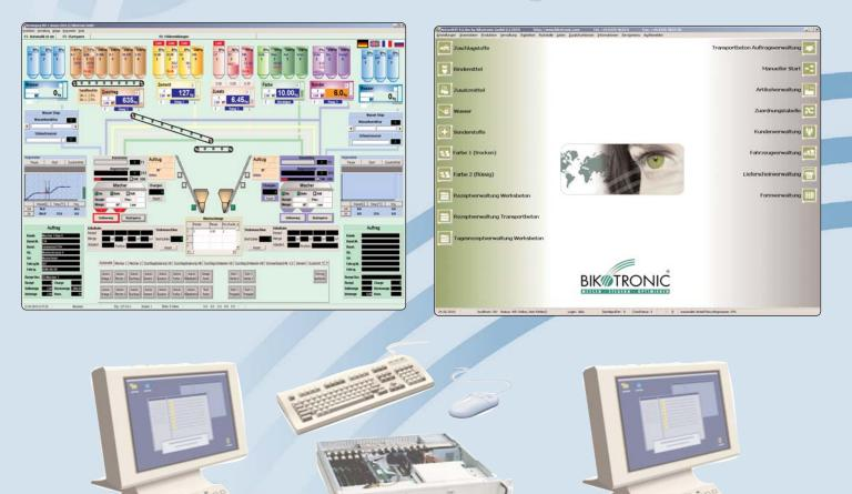
The Beton-WIN SQL System allows the manual and automatic control of the processes in the concrete mixing plant. It is composed of the administration software Beton-WIN SQL, the plant visualisation Visu-WIN, the independent batching computer WD-A and a Recovery Set for restoring data. Thanks to its modular structure a tailor-made plant control can be created. For this, only the hardware and software modules necessary for the specific production process will be compiled.
